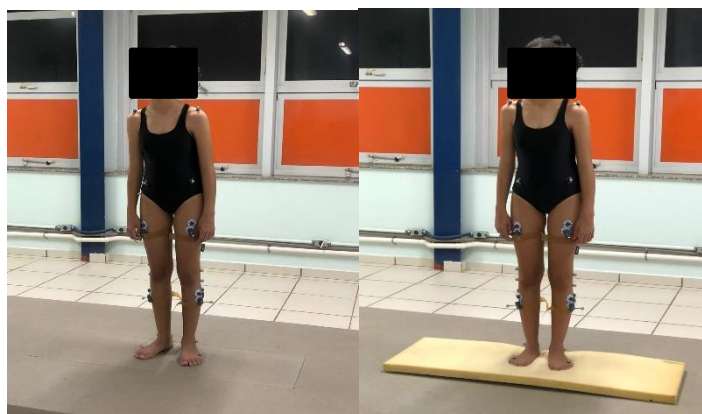
Caption: Patient performing static balance analysis on the Force Platform under two distinct conditions; a) without proprioceptive perturbation; b) with proprioceptive perturbation.
